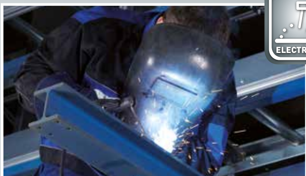
3. MMA / stick electrode welding
