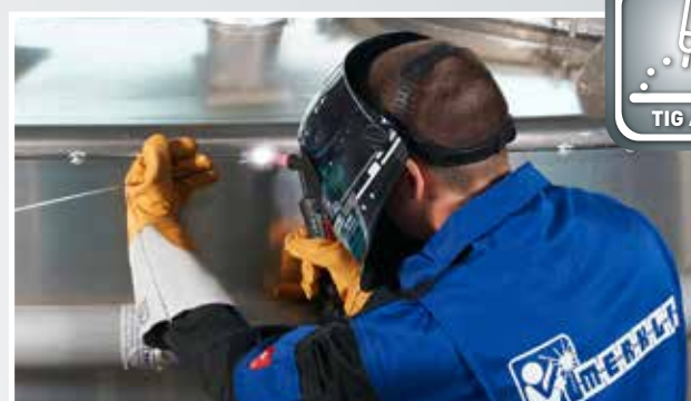
2. Aluminium welding in AC mode (MobiTIG 180 AC/DC)
