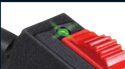
The multi-coloured LED shows the selected energy or program (job).
